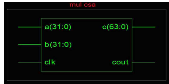
Fig.7. Schematic of 32-bit unsigned CSLA multiplier
